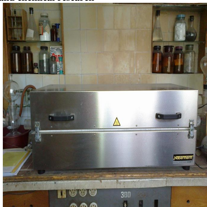
Electric tubular furnace with three zone control
